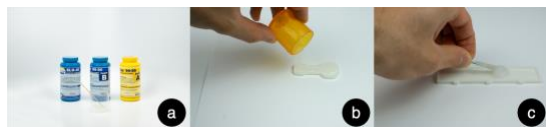
Figure 7: Fabrication. (a) Ecoflex™ 00-50 parts A and B are mixed, (b) poured into the molds, (c) and the top and bottom pieces are then assembled.
